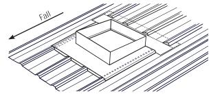
**4.** Refer to SAA HB39 Installation Code for Metal Roofing and Wall Cladding and install accordingly.
