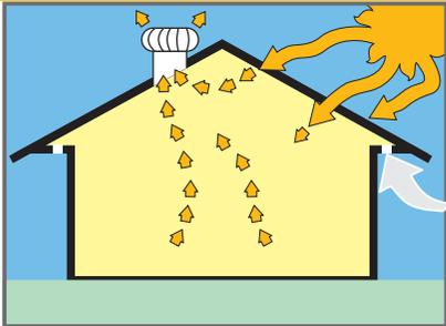
Under eave vents aid roof space air circulation. Install two per Spinaway.
