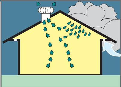
Under eave vents aid roof space air circulation. Install two per Spinaway.
