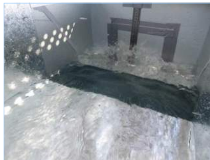
DB 400-1, Q = 16 l/s (box gutter slope - 1 in 200)
