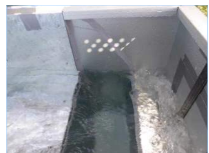
DB 400-1, Q = 16 l/s (box gutter slope - 1 in 200)
